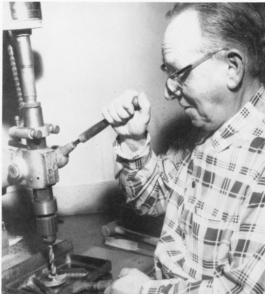
Paul Schoenmehl demonstrates the new holding fixture being used on drill press work in Metals Research. Note the two metal inserts in the pan which form a "V" to wedge the brass sample. As the rotating drill is lowered to the work, the wedges hold the sample steady and keep it from rotating.
